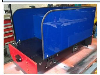
This driving truck is the same as used on our Knight locomotive, built using 12mm frames and 3mm steel superstructure. 6 inch EN8 narrow gauge profile wheels, running in sealed, sprung take-up bearings. Parking brake on one axle.
