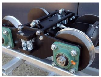
Our heavy duty bogies are designed for the toughest work, weighing in at 27.5kg each. Built for commercial use, these bogies offer excellent track handling and passenger comfort. 6" diameter narrow gauge profile EN8 wheels, sealed self aligning wheel bearings, integrated vacuum braking on all four wheels with mechanical ABS system. These bogies will compensate over the roughest of tracks. Low maintenance and easily adjustable brakes.
