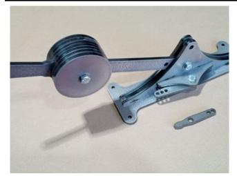
These levers are fully trailable and lockable, laser cut from 6 mm mild steel, this is no light weight! Suitable for use on commercial and club / private tracks. Supplied almost fully assembled with bell crank and also includes a straight arm to allow for optional control methods. Requires handle fitting with supplied single bolt. 30 mm throw and 5 kg pull. Supplied unpainted.
