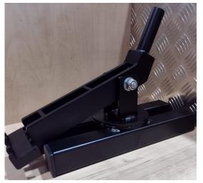
This is the improved design, with wider foot print allowing for both on and off track use. The tool will lift and slew smoothly allowing careful realignment off wheels back onto the track. Can also be used for lifting vehicles for blocking.
