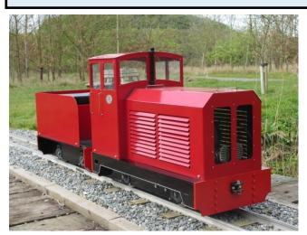
The knight locomotive is a capable medium duty locomotive. Powered by a 6.5hp petrol engine and Eaton hydrostatic transmission.
