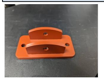
Narrow gauge style single slot coupling block. Laser cut from 6mm mild steel. Supplied assembled and primed.
