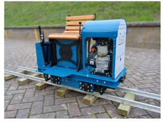
The Scamp is a small 71/4" gauge sit on locomotive. Powered by a petrol engine and two 800watt electric motors. The 1<sup>st</sup> of the motors is driven by the engine and acts as a dynamo, this generated power is used to drive the second motor via a reversing switch and electronic speed controller.
