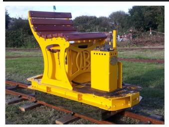
The Flyer is another quirky design from Colin Edmondson. Based on a universal wagon chassis, the Flyer is designed for a bit of fun. Currently supplied as a kit of laser cut parts and wheel sets. A shopping list and instructions are supplied for the other parts required to complete the build, these include a 24 volt 350 watt motor, controller, batteries, and fixings hardware.
