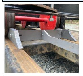
5mm laser cut steel dual scotch to suit both 5" & 6" diameter wheel sets will all metal spreader bar and handle. The scotches are made up of 2 x 5mm plates to give a 10mm thick scotch. These feature pegs to sit inside the rail to aid with fitment avoiding side-to-side movement.
