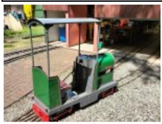
TYKE - 71/4" Sit-in petrol electric / battery electric locomotive. Available as a laser cut kit, including wheelsets, layshafts, machined dynamo pulley and welded bogie pivots.
