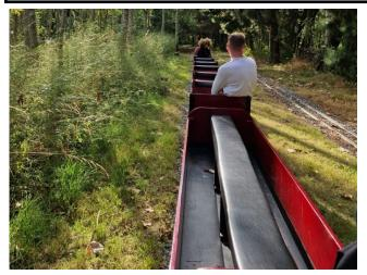
Our standard sit in carriages are built ready to run and come fitted with our heavy duty bogies. Vacuum brakes fitted to one bogie as standard. Heavy duty channel section chassis and ply body . Additional brake sets are optional extras.
